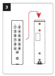
Insert the cable in the hole access area of the back plate. Then mount the keypad on the back plate, placing first the top in the hooks and then the bottom.
