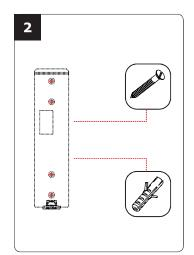
Insert the 2 plastic anchors in the holes. Mount the back plate of the PROFIL100EINT with the screw on the wall.
