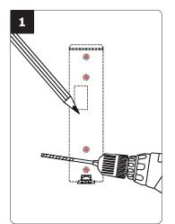
Place the back plate of the PROFIL100EINT on the wall then mark with a pen the hole location then drill the 2 mounting holes (drill bit Ø 5mm a nd 35mm hole depth) and the hole wiring access.
