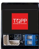
WiFi device for the connection to wind and rain sensors and control of window actuators connected to the WiFi.
